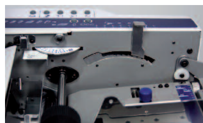
TF MEGA-A: Adjustment of the paper pressure and separation for different paper weights
